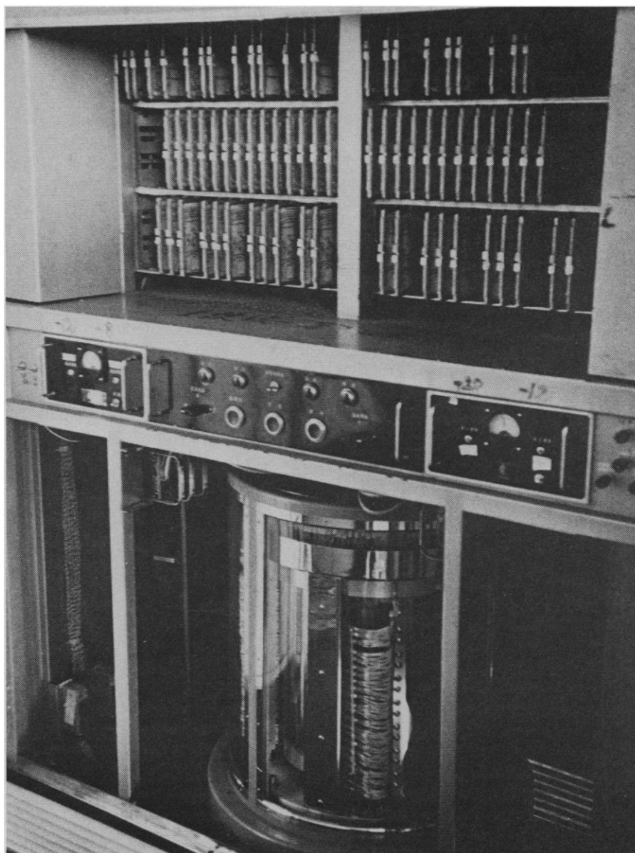
Fig. 5. One of the four magnetic drums of the 109C. Each drum holds 32,048-bit words.
