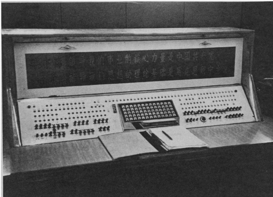
Fig. 3. Console of the 109C at the Peking Institute of Computing Technology. The Chinese inscription is a quotation from Chairman Mao.
