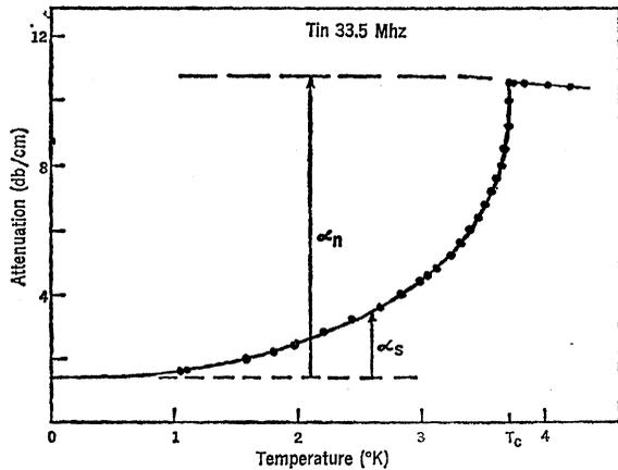
Fig. 8. Ultrasonic attenuation as a function of temperature across the superconducting transition as measured by Morse and Bohm (16). [Courtesy of the American Institute of Physics, New York]
