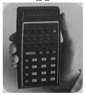
The HP-35 is easier to use, 10 times faster and significantly more accurate than the slide rule. With a single keystroke and in less than a second, it performs trigonometric (sin, cos, tan), logarithmic ( $\log x$ ,  $\ln x$ ,  $e^x$ ) and other commonly used functions ( $x^y$ , 1/x,  $\sqrt{x}$ ,  $\pi$ ) as well as the four arithmetic operations. It also calculates inverse trig functions.
