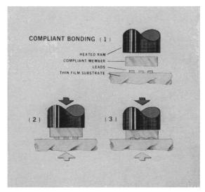
When heat and pressure are applied to the compliant medium, it begins to deform around the gold-plated leads. Deformation of leads is controlled by the flow stress properties of the medium. When the medium bottoms out, it stops the ram and the delicate metal parts are instantaneously and permanently bonded without damage.
