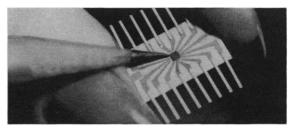
Slightly magnified, the pencil points to a beam-leaded circuit chip which has been bonded to 16 gold conductors that converge on it. Within the silicon chip are dozens of microscopic transistors, diodes, resistors.
