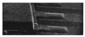
Greatly magnified, we can see gold beam leads projecting from a chip bonded to thin gold conductors on a thin ceramic substrate.
