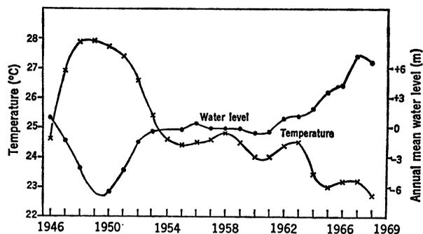
Fig. 2. Variations in annual mean water level and temperature in the crater lake for the period 1946 to 1968. The water level is referred to the datum of 5 April 1946. The drop in water level in the period 1946 to 1950 is a consequence of increased evaporation due to elevated water temperature.
