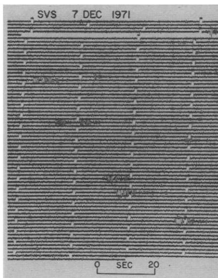
Fig. 8. Part of a seismogram written by the instrument closest to the crater, illustrating the kind of events recorded during the lava eruption. The microseismic background level is about 3 nanometers.
