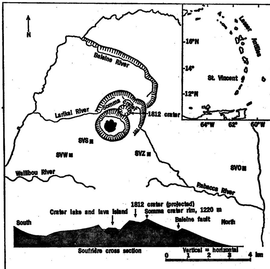
Fig. 1. Schematic map of the Soufrière volcano and the northern part of St. Vincent Island. The cross section is roughly north-south. The black squares indicate the locations of seismograph stations installed during the 1971-1972 eruption.
