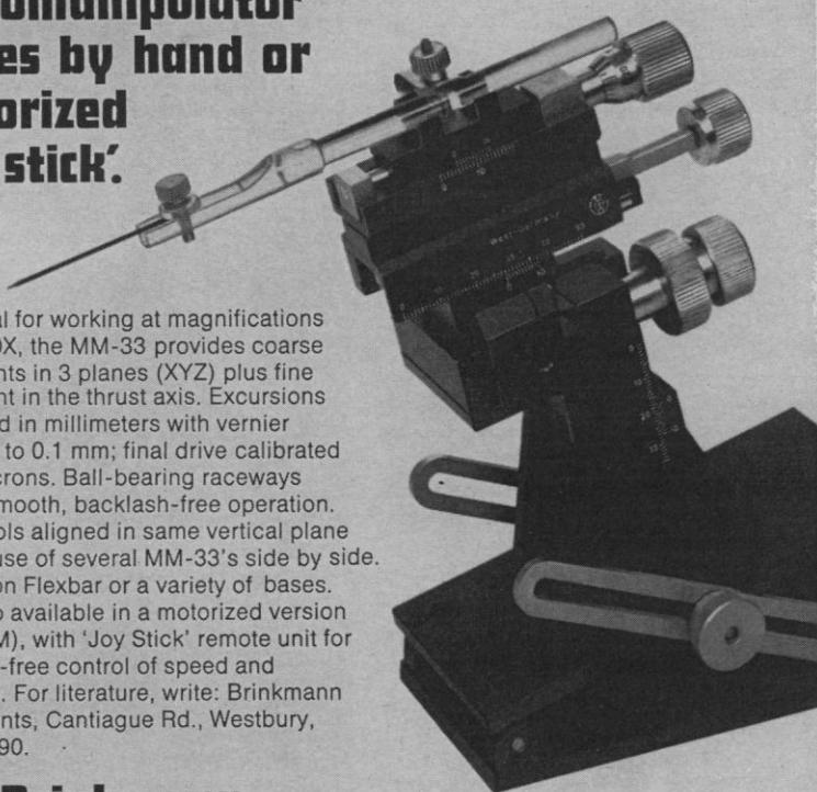
Ideal for working at magnifications up to 250X, the MM-33 provides coarse movements in 3 planes (XYZ) plus fine movement in the thrust axis. Excursions calibrated in millimeters with vernier readings to 0.1 mm; final drive calibrated to 10 microns. Ball-bearing raceways assure smooth, backlash-free operation. All controls aligned in same vertical plane permits use of several MM-33's side by side. Mounts on Flexbar or a variety of bases.
