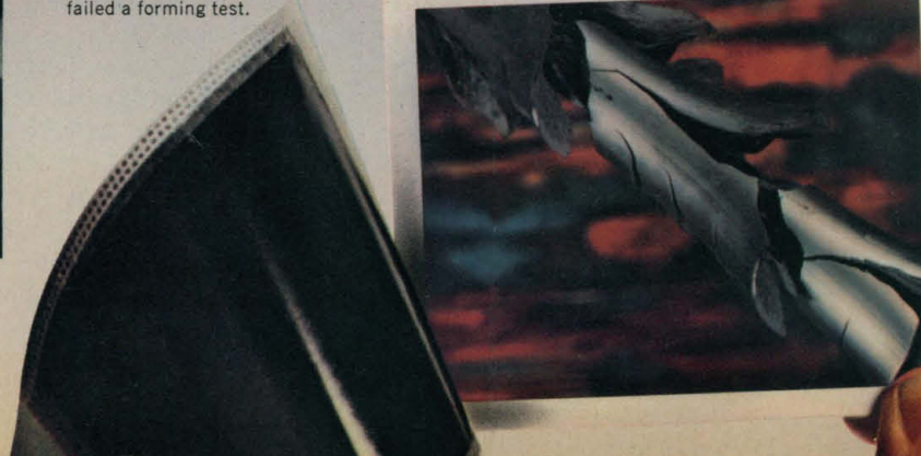
Macrophotography (up to 14.8X). Experimental alloy that failed a forming test.
