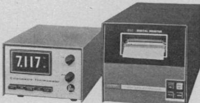
Parr now offers a completely new oxygen bomb calorimeter for measuring the calorific or Brt value of coal, oil, jet fuels, foods and other solid or liquid samples.
