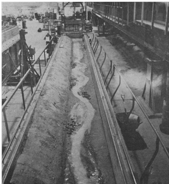
Fig. 1 (left). Downstream view of a sinuous channel in simulated bedrock in the flume at the Hydraulics Laboratory, Engineering Research Center, Colorado State University. Gravel was placed at local low places on the bedrock surface along the channel to prevent overflow at initial bank-full stage. The gravels had no discernible effect on the localization of erosion in the channel. Fig. 2 (right). Transverse profiles of incision through time at two bends (a and c) and the crossing between (b) for the channel shown in Fig. 1. Arrows point to the outside (concave bank) of the bends; distances along the flume are given at each sequence. Stipled areas represent sand deposition; elapsed time is given for each profile in hours.
