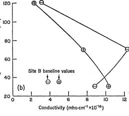
the positive and negative ions were made by simply reversing the polarity of the battery and hence reversing the radial electric field in the sampling tube of the instrument, so the data should have a high relative accuracy and the trends in the profiles should be accurately portrayed even though the absolute conductivities may be in error.
