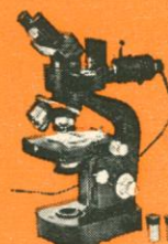
With EPI Attachment for Incident Lighting, Brightfield and Darkfield.
