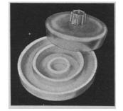
Smooth, white molded polypropylene with natural clear polypropylene cover. Cover has lifting knob and fits annular moat of cell to furnish a positive liquid seal.
