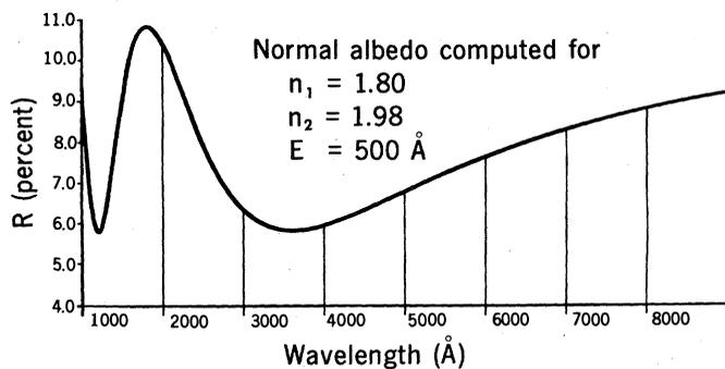
Fig. 3. Reflecting power,  $R$ , of a flat crystalline slab with an index of refraction  $n_2$ , coated with a thin layer (about 500 Å) of metamictized material with an index of refraction  $n_1$  (less than  $n_2$ ), computed as a function of the wavelength. The multielectric structure ( $n_2$  greater than  $n_1$ ),
