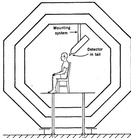
Fig. 1. Magnetoencephalogram (MEG) being taken in the shielded room. For the data presented here the subject's head almost touched the flat end of the Dewar tail and was about 2 cm from the enclosed detector. The detector output, which is proportional to the horizontal component of the magnetic field, goes to an external display station. The subject's clothing must be free of magnetic material, such as zipper fasteners or the nails of shoes.
