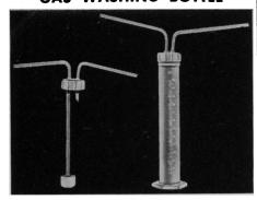
Unbreakable graduated 250 cc polypropylene bottle with tip-proof round base. Top is leakproof screw cap with 1/4" O.D. polyethylene tubes for entrance into gas dispersion chamber and exit for washed gas. Gas is dispersed through porous polyethylene dispersion tube with an average pore size of 35 microns.
