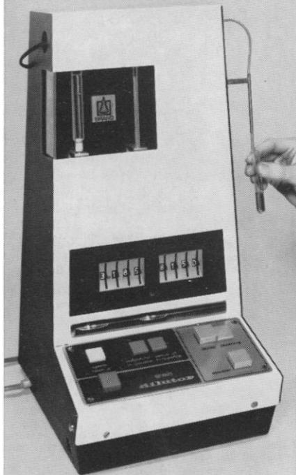
What makes the Brinkmann Automatic Dilutor so expensive (\$2,700) is what makes it so phenomenally accurate: a digital electronic volume setting system, and two precision cylinder and piston assemblies (with only two moving parts in each).
