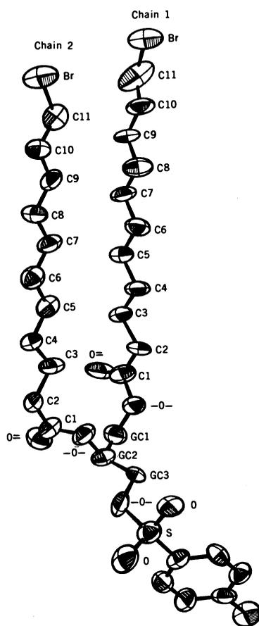
Fig. 1. The molecular structure of *rac* glycerol 1,2-(di-11-bromoundecanoate)-3-(*p*-toluenesulfonate) (**1**).
