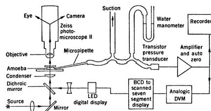
Fig. 1. Block diagram of the experimental arrangement. Abbreviations are: DVM, digital voltmeter; BCD, binary coded decimal output; LED, light-emitting diode. See text and notes for details.
