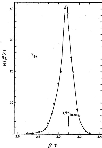
Fig. 3. Spectral line of the  ${}^7\text{Be}$  isotope, uncorrected for energy loss in the target and resolution of the detector-spectrometer system. The arrow indicates the value of  $\beta\gamma$  for the incident  ${}^{14}\text{N}$  beam. The symbol  $\beta$  represents the velocity of the particle divided by the velocity of light, and  $\gamma$  is defined by the equation  $\gamma = (1 - \beta^2)^{-1/2}$ . The ordinate  $N$  is the number of counts observed as a function of  $\beta\gamma$ .
