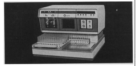
The Automated Pipetting Station from Micromedic Systems is the first instrument that dilutes or dispenses submicro volumes repetitively, automatically, with finer accuracy and technique than manual pipetting. And processes 450 standard test tubes per hour.
