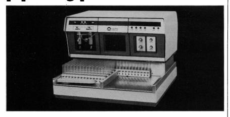
The Automated Pipetting Station from Micromedic Systems is the first instrument that dilutes or dispenses submicro volumes repetitively, automatically, with finer accuracy and technique than manual pipetting. And processes 450 standard test tubes per hour.
