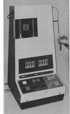
What makes the Brinkmann Automatic Dilutor so expensive (\$2,700) is what makes it so phenomenally accurate: a digital electronic volume setting system, and two precision cylinder and piston assemblies (with only two moving parts in each).
