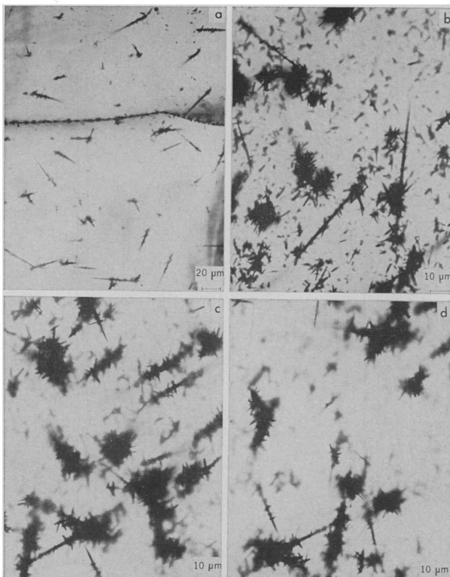
Fig. 5. Long fossil tracks due to VVH nuclei ( $Z \geq 30$ ) in olivine crystal from the Patwar meteorite. (a) Tracks revealed by etching for 20 hours in WN. (b-d) Tracks revealed by etching for 50 hours in WN. A surface layer of 10 to  $30 \mu\text{m}$ , which contained overetched tracks of iron-group nuclei, was removed to obtain a clear view of long tracks. Tracks were decorated with silver for optical contrast according to the method of Macdougall *et al.* (8).
