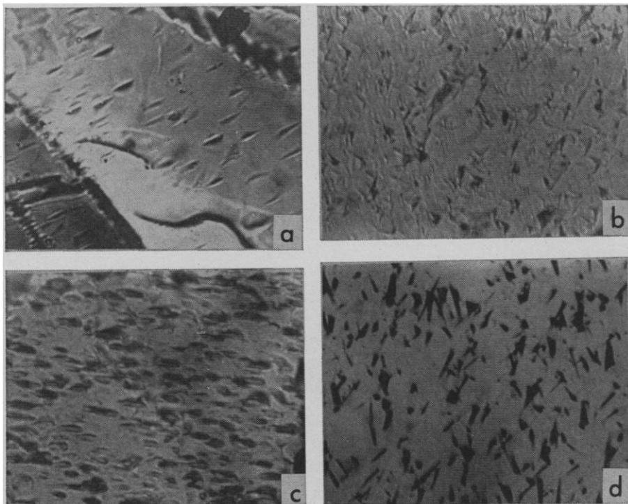
Fig. 2. Solid-state damage patterns in olivines exposed to cosmic-ray nuclei revealed by etching with NaOH or HF. (a) Apollo rock 10017 etched with NaOH (2, 3). (b and c) Patwar meteorite olivines etched with (HF + H<sub>2</sub>SO<sub>4</sub>) (9). (d) Patwar meteorite olivine etched with NaOH (2, 3). The field of view in each of the photographs is approximately 30 by 50  $\mu$ m.
