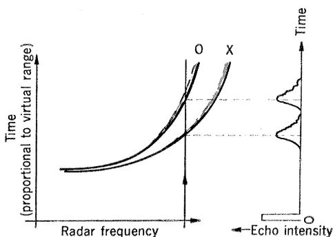
Fig. 8. A demonstration of ionogram synthesis. At the right is a plot of echo intensity versus time delay for a single frequency, and the ionogram at the left is produced by the superposition of such information as a function of frequency, with the echo-intensity information used to modulate the intensity of the oscilloscope trace. The traces on the ionogram are spread, to illustrate the phenomenon of spread F.
