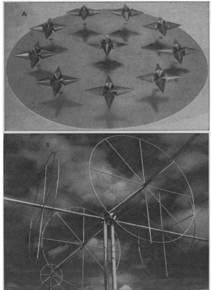
Fig. 2. (A) A model of the 5- to 10-megahertz crossed-dipole antenna array at Platteville, constructed to a scale of 1:100. The nine-element ring has a diameter of 110 meters in the full-scale array. The central element aids in suppressing side lobes. (B) A portion of one element of the actual antenna array at Platteville.
