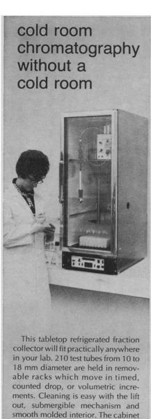
smooth molded interior. The cabinet has a brushed stainless steel exterior and double pane full size glass door. Columns with a maximum length of 1 meter can be clamped to removable sliding wire racks, which also hold buffer reservoirs, pumps, and general cold storage items.
