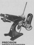
REFRACTOMETER High precision with ability to measure at any wavelength. Overall range: 1.20-1.70N<sub>D</sub>.
