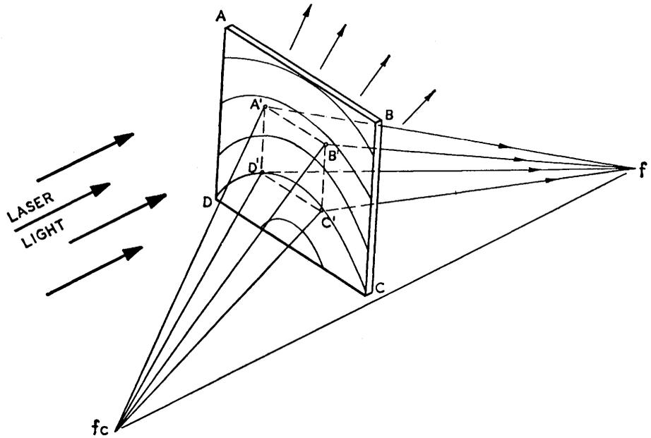
Fig. 9. Only a part of a hologram is necessary to reconstruct a scene in its entirety. [After (5)]
