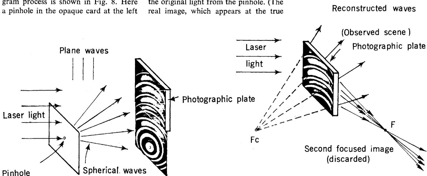
Fig. 8. Circular interference fringes, corresponding to a zone plate, are created by the interference pattern formed by plane waves arriving from left and by spherical waves emerging from the pinhole. If a portion of this pattern is recorded on a photographic plate, the resulting hologram, when illuminated, causes waves to be generated, and reconstructs the image as if it came from the original location of the pinhole. [After (5)]
