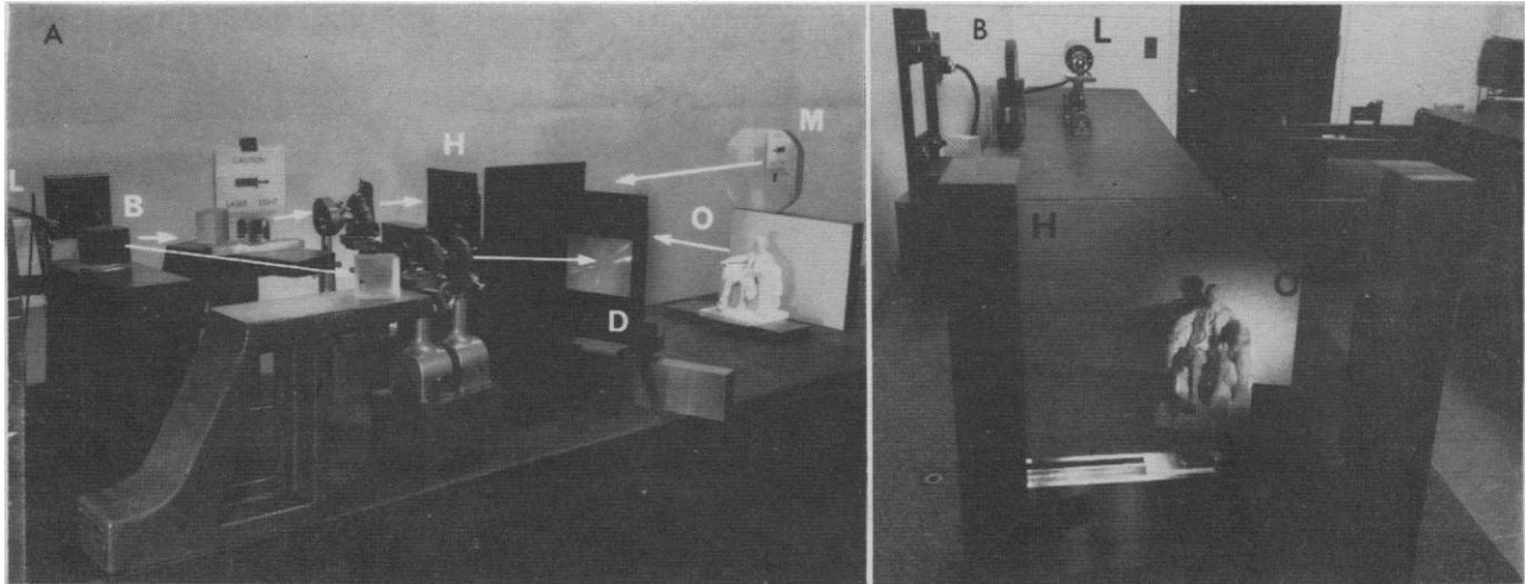
Fig 2. (A) Experimental arrangement for the recording of a three-dimensional hologram. *L*, laser; *B*, beam-splitting mirror; *M*, reference mirror; *D*, diffusor for diffuse illumination of object *O*; *H*, hologram (photographic plate). (B) View through hologram *H* recorded in arrangement of A. [After (4)]
