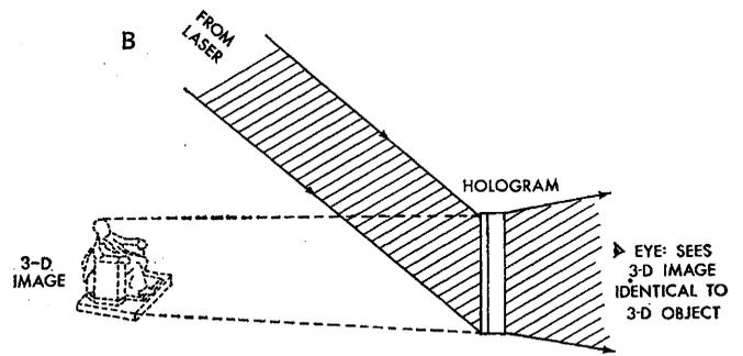
Fig. 1. (A) Hologram recording arrangement. (B) Holographic image reconstruction arrangement.
