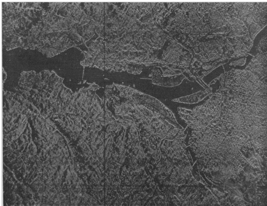
Fig 13. Photographic image of Washington, D.C., extracted by laser light illumination from a photograph of an oscillograph display of a microwave hologram (such as that of Fig. 12) recorded according to the method of (17). [Courtesy of L. J. Cutrona *et al.* (19), see also (20-25)]
