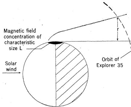
Fig. 1. Trace of the limb shock due to a region of permanent magnetic field on the plane of the orbit of Explorer 35.
