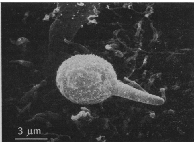
Fig. 1 (left). Fibers of methyl 2-cyanoacrylate polymer. Fig. 2 (right). Fiber which developed a ball at its tip after divinyl sulfone vapor was added to the flow of methyl 2-cyanoacrylate vapor.
