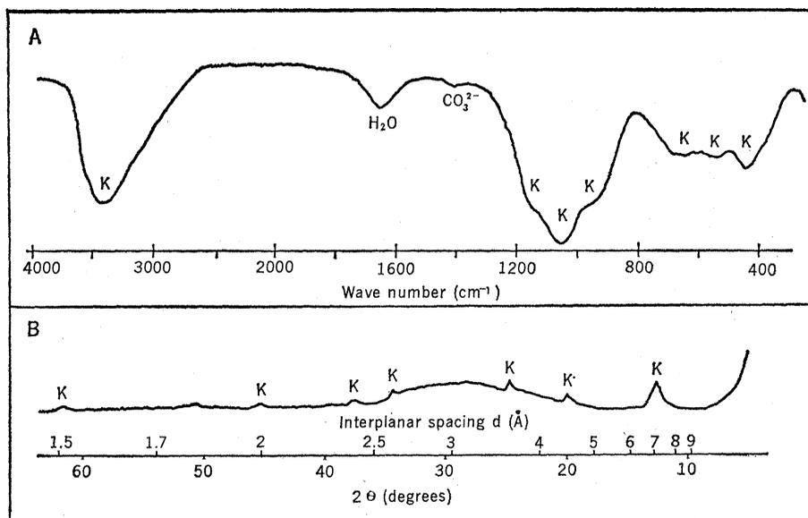
Fig. 2. (A) Infrared spectrum and (B) x-ray diffraction pattern of a synthetic kaolinite ( $pH = 7$  and  $SiO_2/Al_2O_3$  ratio in solution = 2).
