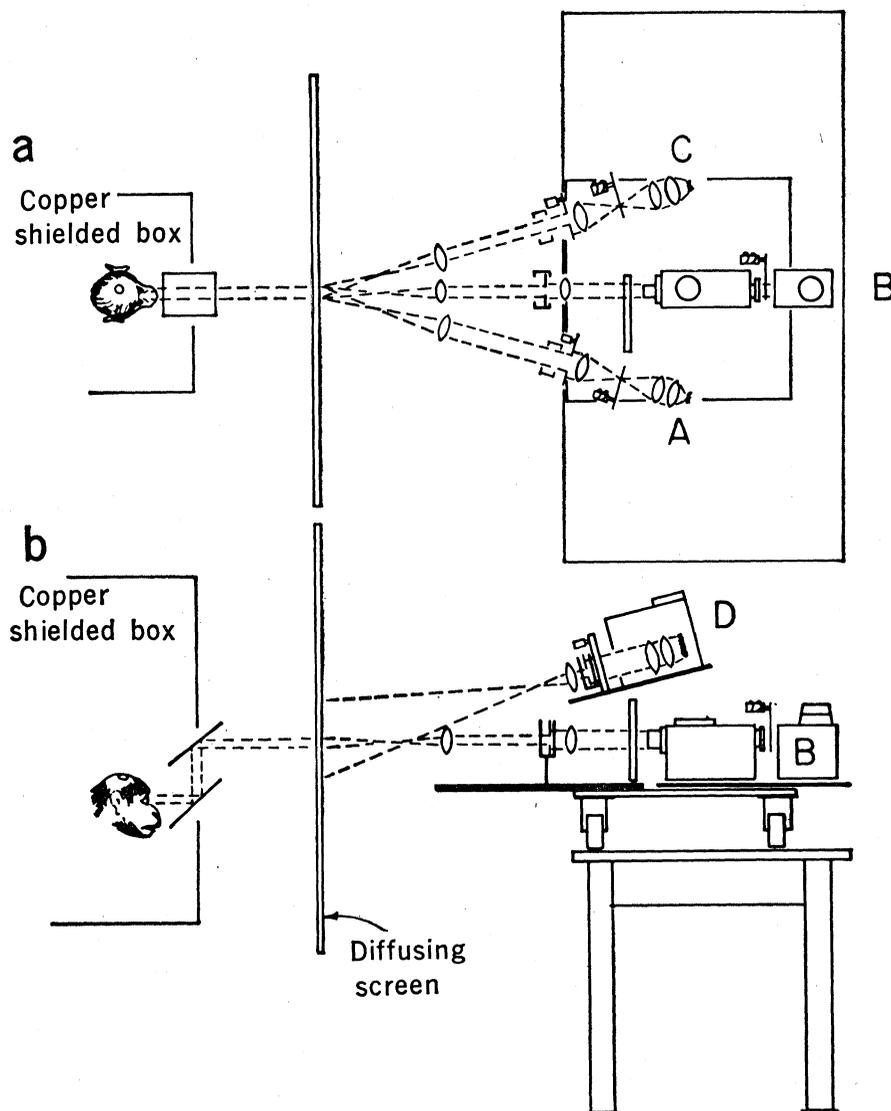
Fig. 1. Diagram of the optical system used. (a) Top view; (b) side view.
