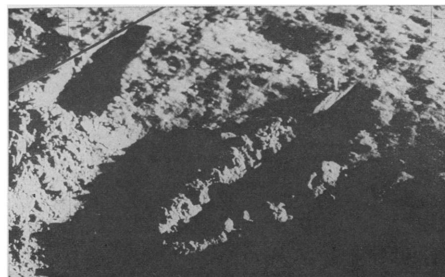
Fig. 2. Part of Apollo 12 photograph, taken 20 November 1969, showing trenches made by Surveyor 3 surface sampler. Far corner of nearer trench preserves vertical wall, about 6 cm deep, dug 22 April 1967. From photograph AS 12-48-7108.
