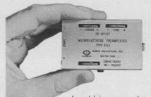
Input bias current: <1 x 10<sup>-12</sup> amps@ 25°C. Input offset current: 1 x 10<sup>-12</sup> amps@ 25°C.
