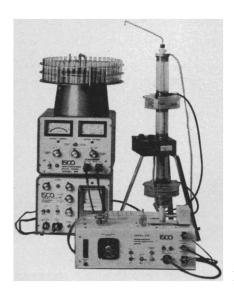
Easy determination of electrophoretic mobilities as well as physical separation of mixtures and quantitative microanalytical results can be obtained with the ISCO Model 210 Density Gradient Electrophoresis apparatus. Microgram size samples can readily be separated. Low sample concentration permits the use of dilute buffers, allowing a wide operational temperature range of from 0 to 25° C.
