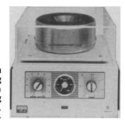
nal or other body fluids. Centrifugation and slide preparation are performed simultaneously, which eliminates prior centrifugation and saves you time. Improved head design ensures safety when working with pathogenic organisms.
