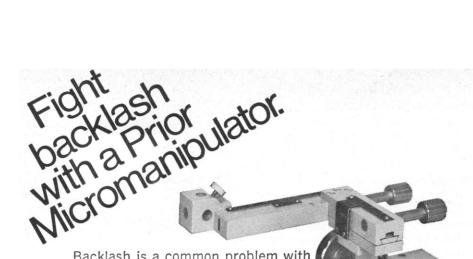
Backlash is a common problem with many micromanipulators, but not with a Prior. Its robust, worm-drive movement always remains exactly as set. The Model 20 shown here features extremely precise fine adjustment; a complete rotation of the calibrated fine adjustment knob moves the slide only .127 mm. The Prior 20 may be ordered with right or left-hand controls, fixed or tilting arm, and a variety of bases. Microdrive attachments, needle holders and other accessories are available.
