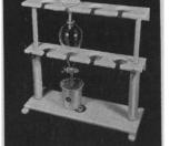
**SEPARATORY FUNNEL RACK** Adjustable in height for 4 separatory funnels.
