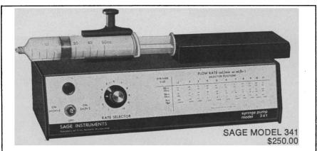
This new single-channel syringe pump gives you a choice of 132 easy-to-set flow rates from .092  $\mu$ l/hr to 13 ml/min. The Sage Model 341 accepts all types of syringes, any size from the smallest microliter to 50 cc. With any given syringe, you get a flow rate range of 2,350 to 1. Flow rates – all shown on the control panel – are precalibrated, highly reproducible and constant. New universal syringe holder and easily-set selector switch make set-up and operation swift and sure.
