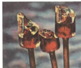
Diode fractures, for QC report. Polacolor Type 108 film.
