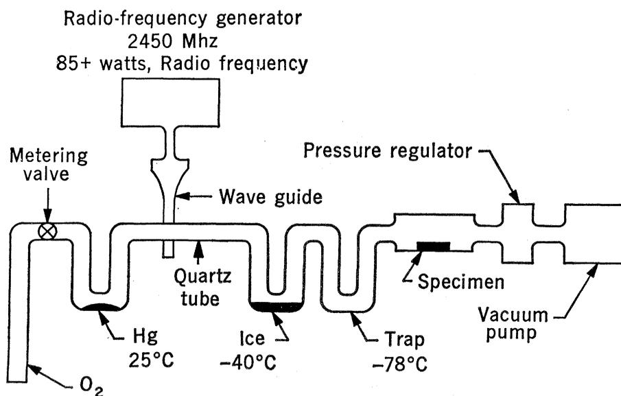
Fig. 1. Diagrammatic representation of the flow system used for polymer oxidation.
