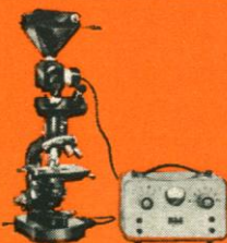
With Binocular Camera Lucida, the first of its kind; up to 1:5 enlargement ratio.
