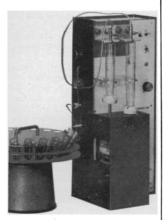
The ISCO Model 570 is a fully automatic instrument for forming sucrose, CsCl, or other density gradients used in density gradient ultracentrifugation and electrophoresis. Convex, concave, linear, and exponential gradients from 3 to 80 ml can be programmed without cutting any cams. All gradients are identical and faithful reproductions of the desired curve.
