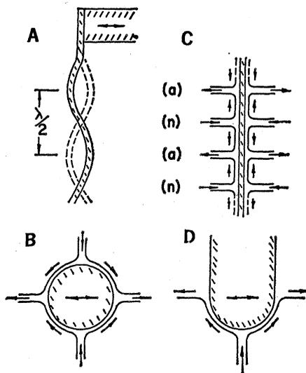
Fig. 2. Schematic of vibrating wire device and circulatory patterns. (A) Attachment of wire to driver. (B) Streaming as it occurs near a transversely oscillating rigid cylinder in plane perpendicular to axis. Arrows near boundary show  $U_L$ . (C) Streaming associated with flexural vibrations of wire in the plane of vibration; displacement nodes are at  $n$ , and antinodes are at  $a$ . (D) Streaming associated with the tip in plane of vibration.
