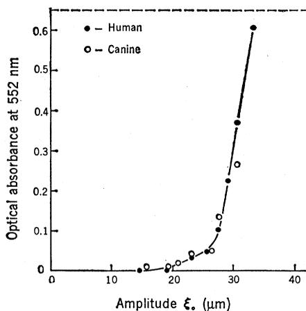
Fig. 1. Hemoglobin release from erythrocytes in suspension, brought about by a partially immersed tungsten wire set into transverse vibration for 5 minutes at a frequency of 20 khz. Osmotic hemolysis in distilled water yields an absorbance value of 0.65, as shown by dashed line.
