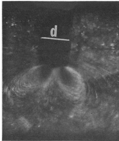
Fig. 1. Bubble-associated streaming pattern obtained by timed-exposure of side-lighted polystyrene spheres (7 to 14  $\mu\text{m}$  in diameter). Amplitude  $\xi_0$  is 26  $\mu\text{m}$ . Dimension  $d$  shown on photograph gives the tube diameter (520  $\mu\text{m}$ ). See Fig. 2 insert for line drawing of arrangement.
