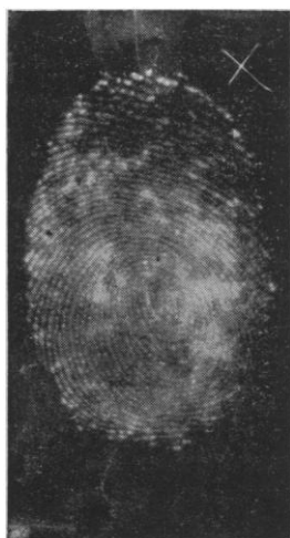
Fig. 1. Autoradiograph of a thumbprint on a zinc borosilicate glass slide after adsorption of 14 C-labeled stearic acid from benzene solution and subsequent partial desorption with 1,1,2-trichlorotrifluoroethane. Industrial x-ray film was used with an exposure time of 120 hours.
