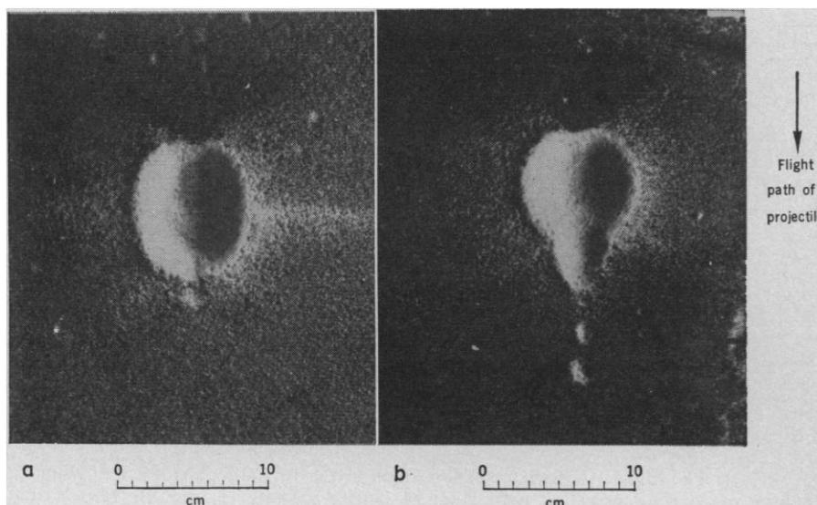
Fig. 1. Photographs of experimental craters in sand illustrating the extremes in morphological forms produced. A thin layer of dyed sand was placed over silica sand to enhance the contrast. Forms range from (a) elliptical craters to (b) doublet craters. Intermediate cases between these extremes were also observed. Note the well-developed side lobes in the ejecta surrounding the craters.
