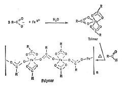
On heating, the sticky resin is changed into a hard, glassy material which breaks with conchoidal fracture. Metals other than iron which yield these polymers include cobalt, copper, nickel, titanium, manganese, and chromium. The nature of the R-group on the aldehyde is not critical. However, it has been found that if the R-group on the aldehyde is similar to the R-group on the acid, the reaction proceeds more readily.
