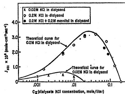
Fig. 2. Flow of KCl as a function of dialysate KCl concentration. The curves are calculated for dialysand concentrations of 0.2 and 0.02M KCl, with  $(R_c + R_a)$  assumed to be 13.1 ohm-cm<sup>2</sup>. The points are experimental.
