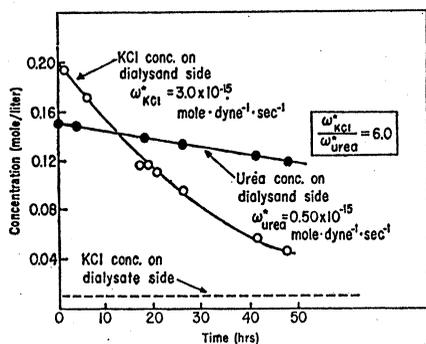
Fig. 1. Diallytic separation of KCl from urea by means of a charge-mosaic membrane. The permeability  $\omega_{KCl}^*$  is that obtaining with 0.1M KCl in the dialysand.
