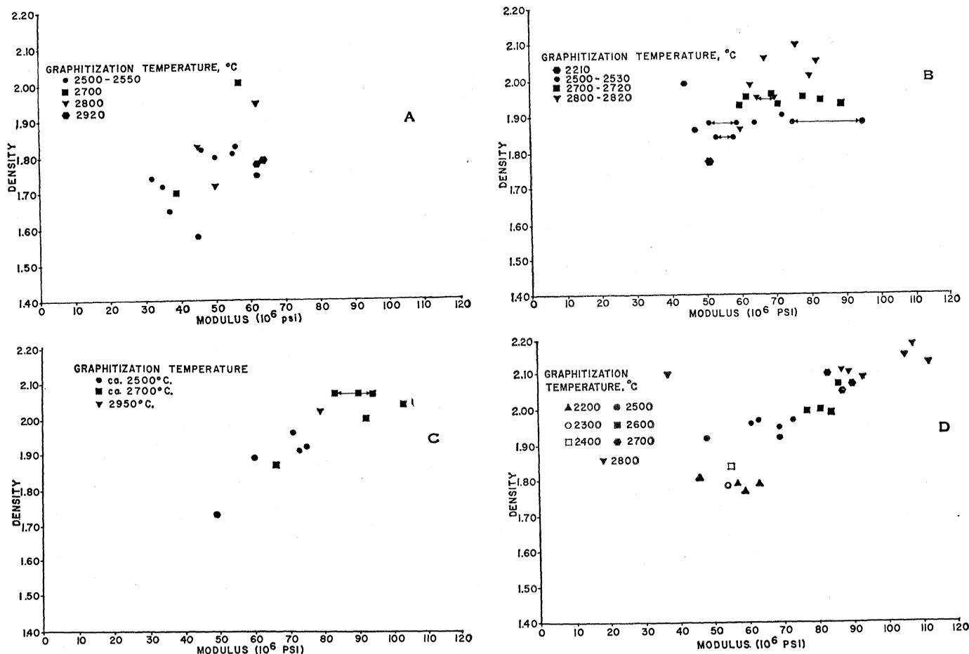
Fig. 1. Density (g/cm<sup>3</sup>) and modulus values for graphite fibers from acrylic precursor yarns. (A) Courttelle, (B) PAN, (C and D) Dralon T.
