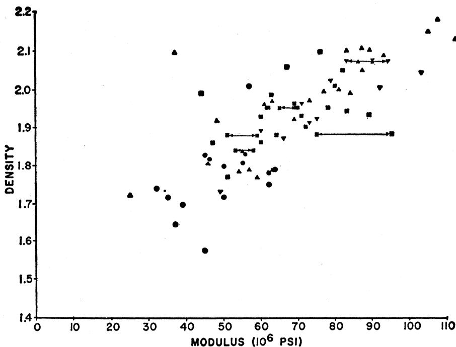
Fig. 2. Density ( $\text{g}/\text{cm}^3$ ) and modulus values for graphite fiber samples from all of the acrylic precursors: (●) Courtelle, (■) PAN, (▲ and ▼) Dralon T.
