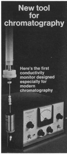
This new monitor detects conductivity as low as .001  $\mu$ mho (.01 ppm NaCl) using a flow-through cell with only 1.5 microliters volume. Response is linear at the recorder output over a million-to-one range from .001 to 1000  $\mu$ mhos.
