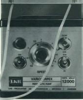
The VarioPerpex has continuously variable flow rates within the wide range 1.6 to 200 ml per hour, for a standard gear box, and lower flow rates are possible by using other easily exchangeable gear boxes. Fluctuations, due to mains voltage variations, have been reduced to a minimum by the employment of a stepmotor.
